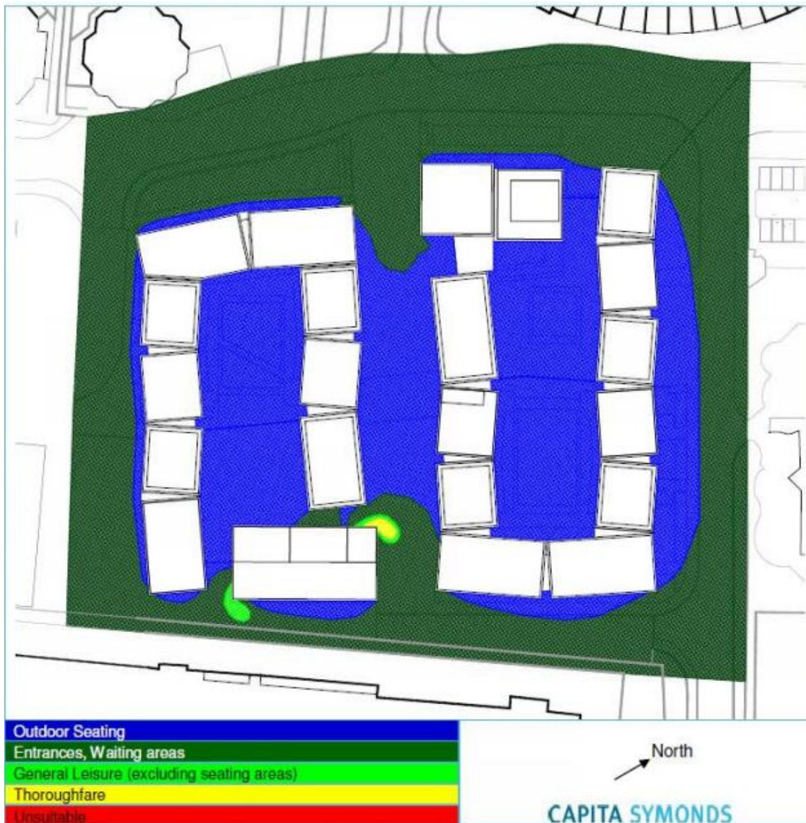
Image above: Wind conditions created by the 2013 planning permission (current baseline conditions)
